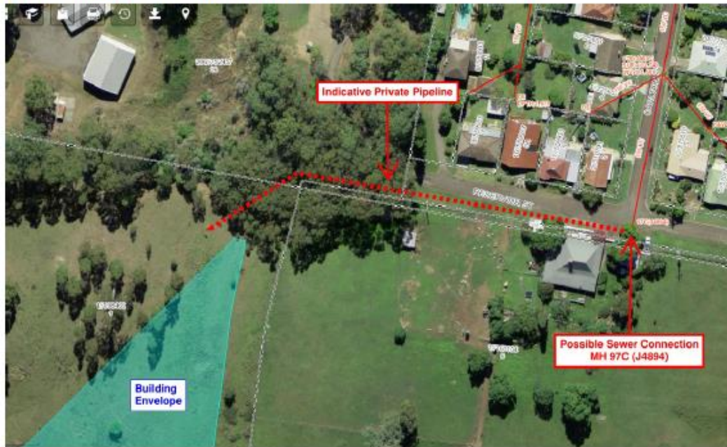
Figure 2: Possible Sewer Connection for Private Pump to Sewer System
